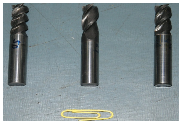
Fig.3: Endmills used in the experiment (50°, 27°, 38° Helix angles)
